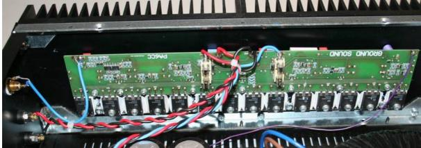
The **input** wiring should be made with shielded cable – only one inner core is required for unbalanced RCA connector.
